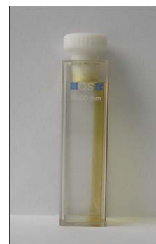
Fig. 3 Thin film of HPG2 adsorbed on a wall of a fluorescence cuvette. Kinetic runs can be spectrophotometrically monitored through the clean area of the front window.
